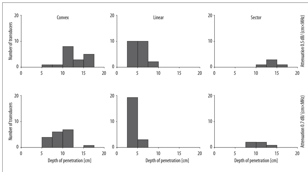
**Figure 2.** Results of the depth of penetration test.
